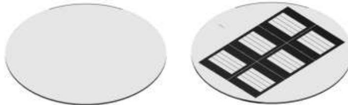
Figure 3. Aperture definition by structured coating of a low reflective chromium (LRC) mask
