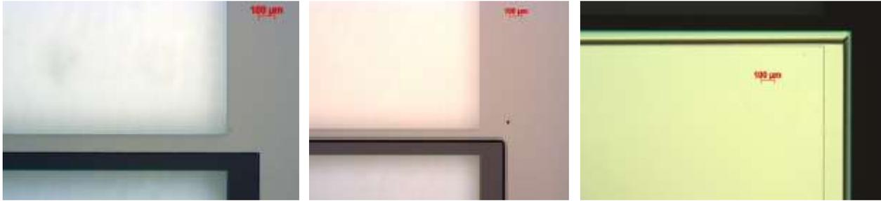
Figure 6. Dimensional transformation of a  $\sim 9\mu\text{m}$  photoresist/coating system from resist (left), treated resist (center) to final filter after coating and lift-off (right)
