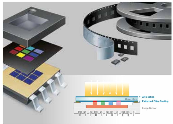
Sensor Package for Ambient Light Sensing
