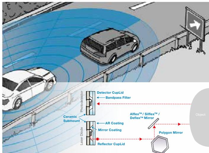
Scanning LiDAR with Polygon Mirror
