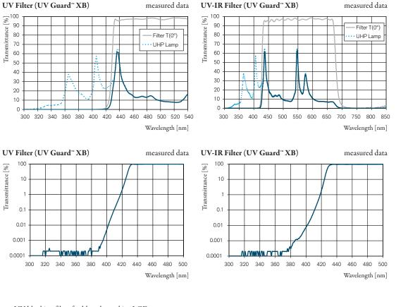
UV-blocking filter for blue channel in tLCD Primary UVIR filter with extreme UV-blocking for tLCD/ LCOS UV blocking filter with broadband RGB transmission
