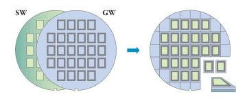
Schematic Wafer Level Packaging: Entire semiconductor wafer (SW) with array of sensors is covered by a cover glass wafer (GW) – see left side. Combined wafers are cut into pieces (right side).
