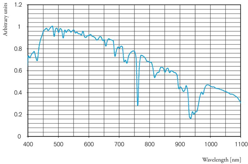
**Customer specific solar filter for extended wavelength range UV-IR**
