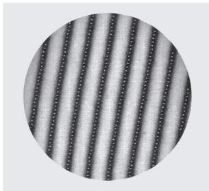
Interferogram of surface flatness
